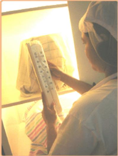
**7. Checking the temperature:** The temperature of the culturing cabinet is regularly checked and maintained at 35-38 degrees Celsius.
