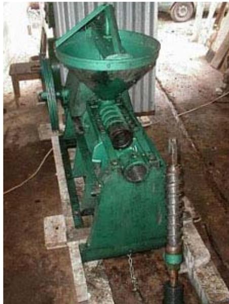
The large hopper is where the dried gratings are dropped in and fed to the screw expresser. The hanging sheet of metal separates the prime drive from the expresser. The two are connected by 10 foot long drive belts. The primer mover is Lister Diesel "copy" made in India. They first built these style engines in England in the late 1800's and stopped
