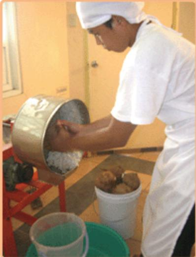
**3. Grating:** Using a motor-powered grater, coconut meats are grated into fine strands.
